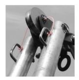
This pulley can now be dismantled easily to fit the rope every time it is used without removing the legs.
